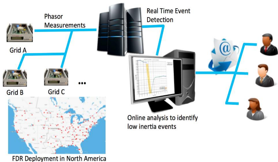
Figure 1-9. FNET/GridEye real-time low inertia detection implementation.
