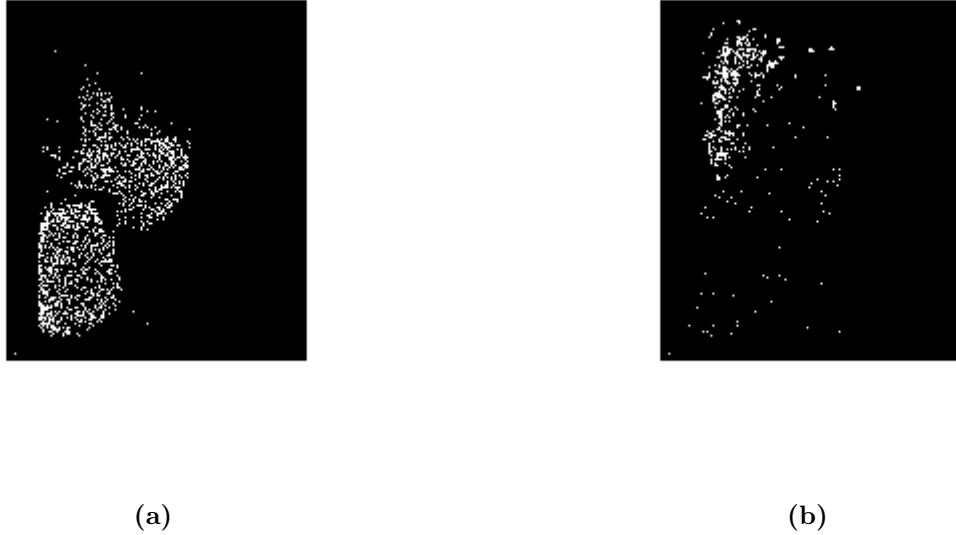
Figure 6.13: (a) Dark field and (b) Knife edge images for the Timepix-coupled LISe sensor for 9 MeV neutron exposure.
