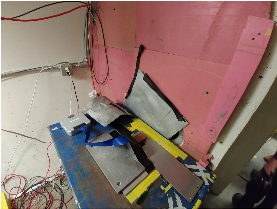
Figure 5.21: Image of the experimental setup with the detector. The collimation port and detector were covered with a thin layer of Cd to eliminate moderated thermal neutrons.
