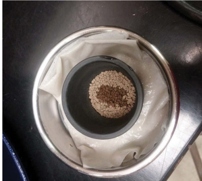
Figure 1.1. Soil samples were allowed for a gradual capillary absorbnce of water from the bottom of sieve to avoid the air entrapment.
