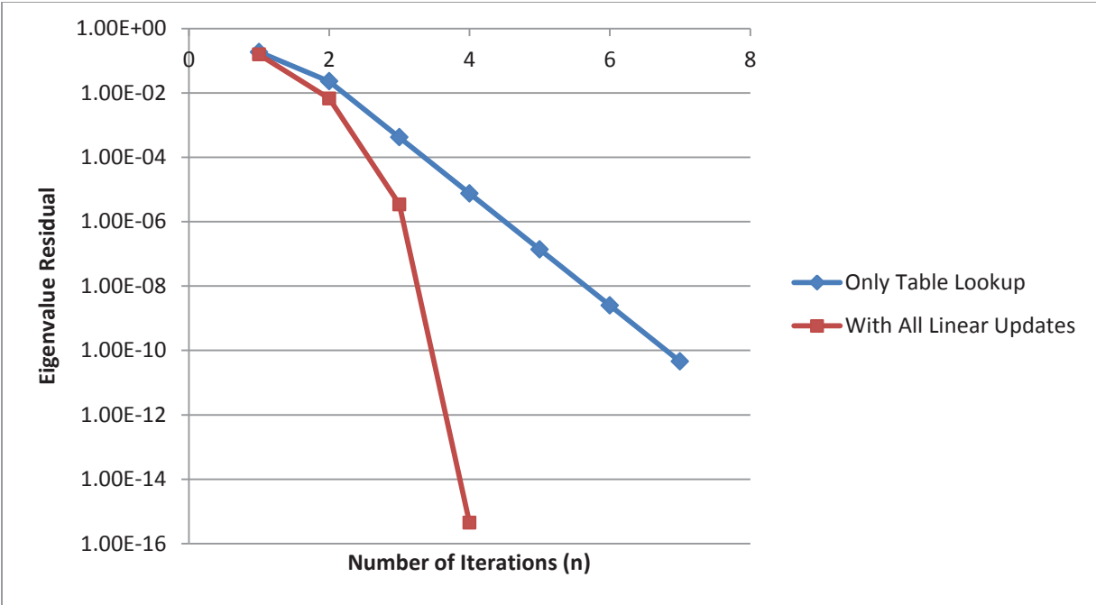
Figure 5. Convergence of a table lookup (Algorithm 6) vs the addition of a linear update
