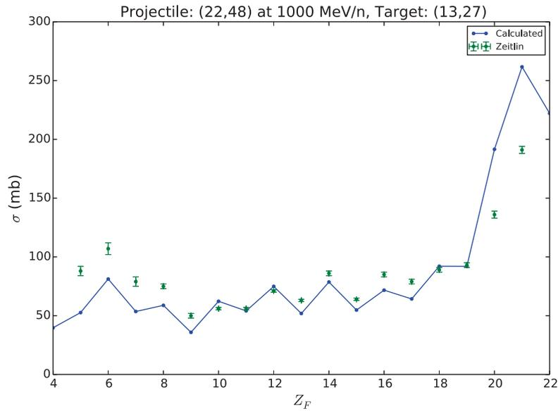
**Figure 4.50:** Elemental production cross sections (solid) compared with experimental measurements (error bars) from Ref. [54] for the reaction of  $^{48}\text{Ti}$  on  $^{27}\text{Al}$  at 1000 MeV/A.
