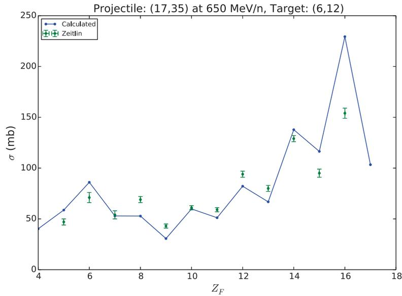
**Figure 4.24:** Elemental production cross sections (solid) compared with experimental measurements (error bars) from Ref. [54] for the reaction of  $^{35}\text{Cl}$  on  $^{12}\text{C}$  at 650 MeV/A.
