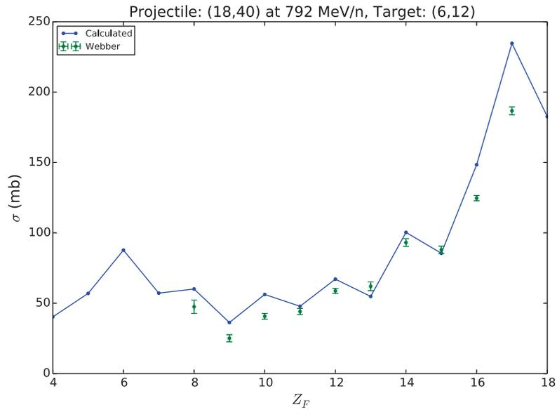
**Figure 4.48:** Elemental production cross sections (solid) compared with experimental measurements (error bars) from Ref. [48] for the reaction of  $^{40}\text{Ar}$  on  $^{12}\text{C}$  at 792 MeV/A.
