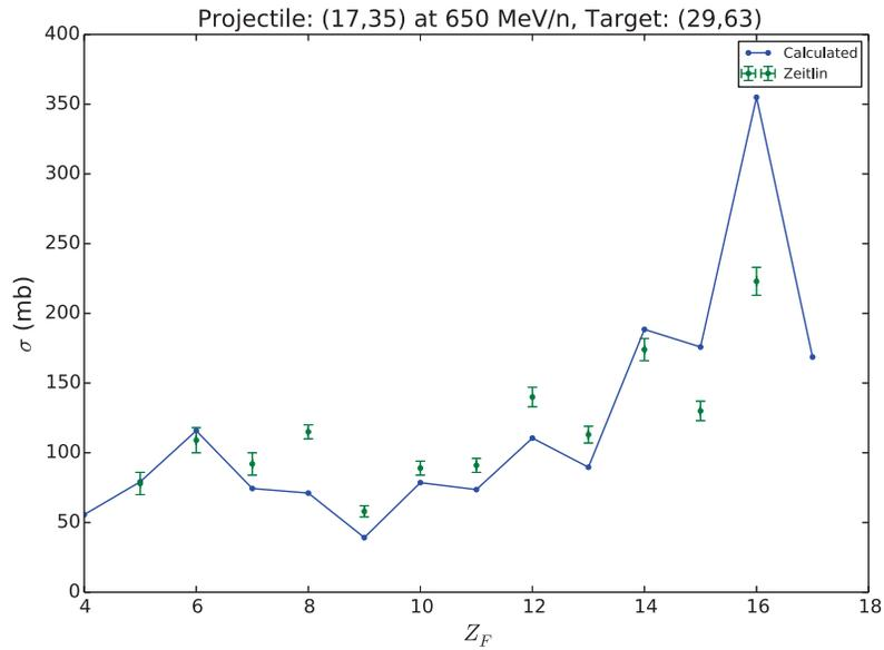
**Figure 4.26:** Elemental production cross sections (solid) compared with experimental measurements (error bars) from Ref. [54] for the reaction of  $^{35}\text{Cl}$  on  $^{63}\text{Cu}$  at 650 MeV/A.
