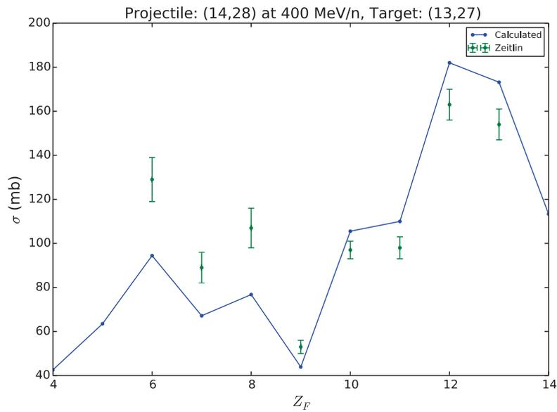
**Figure 4.22:** Elemental production cross sections (solid) compared with experimental measurements (error bars) from Ref. [52] for the reaction of  $^{28}\text{Si}$  on  $^{27}\text{Al}$  at 400 MeV/A.
