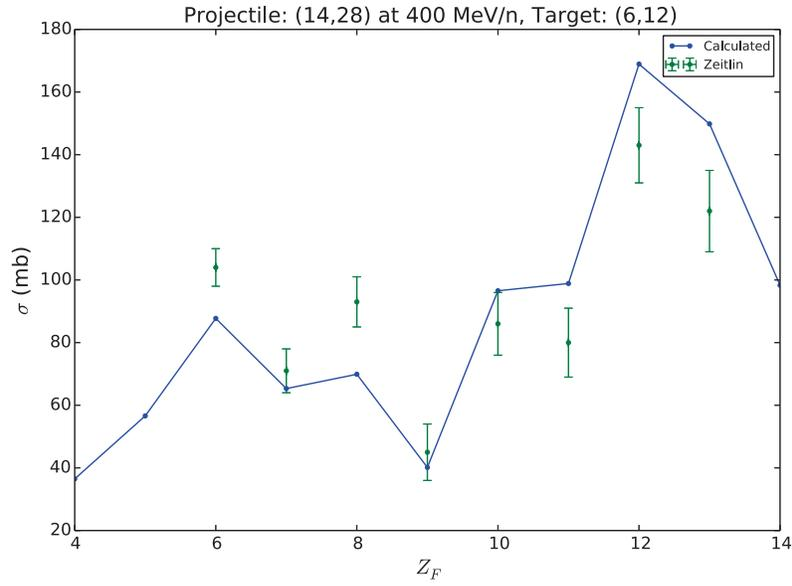
**Figure 4.21:** Elemental production cross sections (solid) compared with experimental measurements (error bars) from Ref. [52] for the reaction of  $^{28}\text{Si}$  on  $^{12}\text{C}$  at 400 MeV/A.
