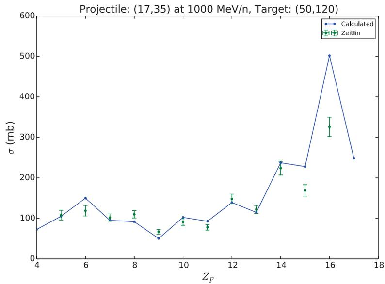
**Figure 4.32:** Elemental production cross sections (solid) compared with experimental measurements (error bars) from Ref. [54] for the reaction of  $^{35}\text{Cl}$  on  $^{120}\text{Sn}$  at 1000 MeV/A.
