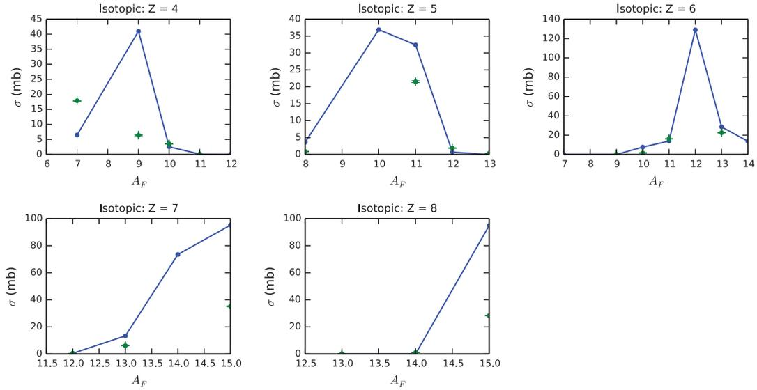
**Figure 4.54:** Isotopic production cross sections (solid) compared with experimental measurements (error bars) from Ref. [55] for the reaction of  $^{16}\text{O}$  on  $^{12}\text{C}$  at 290 MeV/A.
