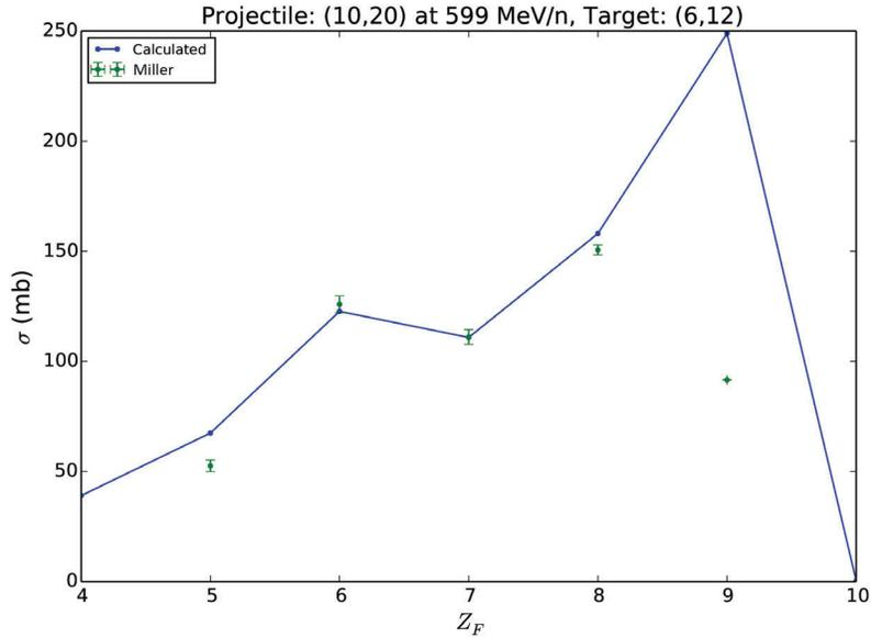
**Figure 4.16:** Elemental production cross sections (solid) compared with experimental measurements (error bars) from Ref. [29] for the reaction of  $^{20}\text{Ne}$  on  $^{12}\text{C}$  at 599 MeV/A.
