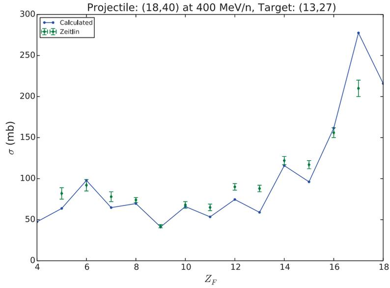
**Figure 4.45:** Elemental production cross sections (solid) compared with experimental measurements (error bars) from Ref. [54] for the reaction of  $^{40}\text{Ar}$  on  $^{27}\text{Al}$  at 400 MeV/A.
