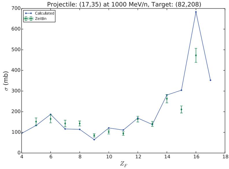
**Figure 4.33:** Elemental production cross sections (solid) compared with experimental measurements (error bars) from Ref. [54] for the reaction of  $^{35}\text{Cl}$  on  $^{208}\text{Pb}$  at 1000 MeV/A.
