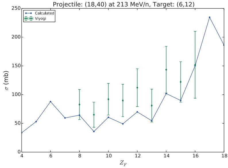
**Figure 4.37:** Elemental production cross sections (solid) compared with experimental measurements (error bars) from Ref. [47] for the reaction of  $^{40}\text{Ar}$  on  $^{12}\text{C}$  at 213 MeV/A.
