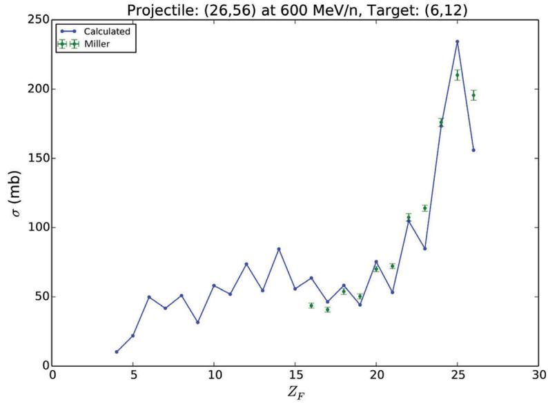
**Figure 4.51:** Elemental production cross sections (solid) compared with experimental measurements (error bars) from Ref. [29] for the reaction of  $^{56}\text{Fe}$  on  $^{12}\text{C}$  at 600 MeV/A.
