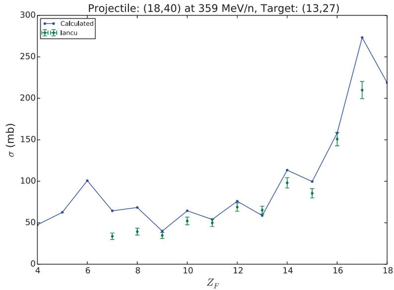
**Figure 4.42:** Elemental production cross sections (solid) compared with experimental measurements (error bars) from Ref. [18] for the reaction of  $^{40}\text{Ar}$  on  $^{27}\text{Al}$  at 359 MeV/A.
