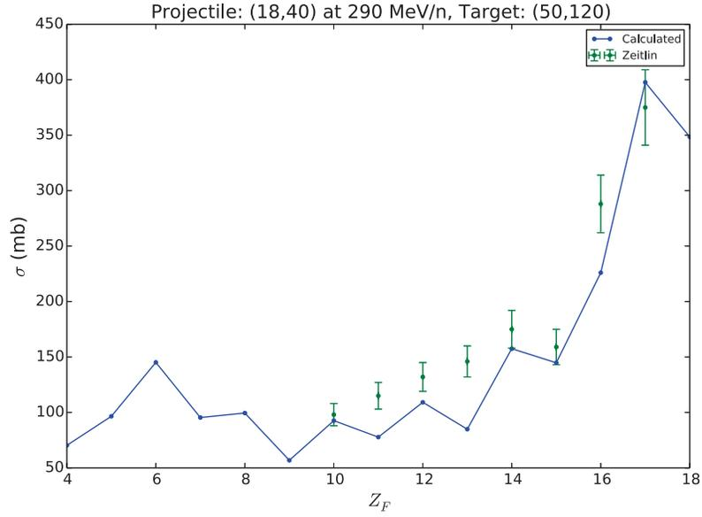
**Figure 4.41:** Elemental production cross sections (solid) compared with experimental measurements (error bars) from Ref. [54] for the reaction of  $^{40}\text{Ar}$  on  $^{120}\text{Sn}$  at 290 MeV/A.
