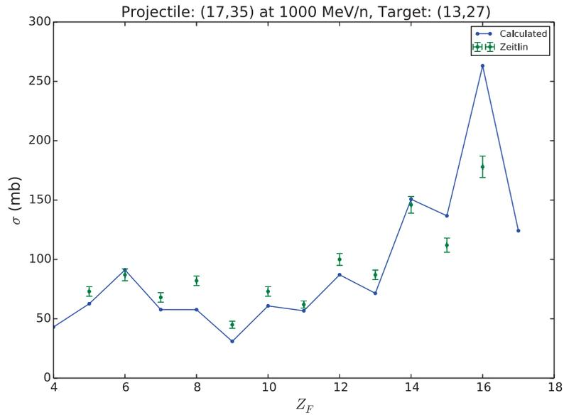
**Figure 4.30:** Elemental production cross sections (solid) compared with experimental measurements (error bars) from Ref. [54] for the reaction of  $^{35}\text{Cl}$  on  $^{27}\text{Al}$  at 1000 MeV/A.
