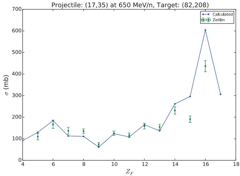
**Figure 4.28:** Elemental production cross sections (solid) compared with experimental measurements (error bars) from Ref. [54] for the reaction of  $^{35}\text{Cl}$  on  $^{208}\text{Pb}$  at 650 MeV/A.
