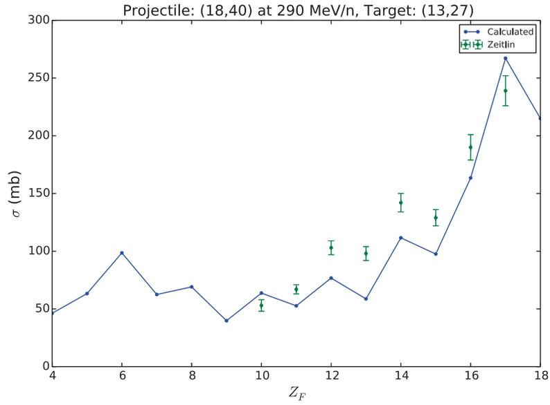
**Figure 4.39:** Elemental production cross sections (solid) compared with experimental measurements (error bars) from Ref. [54] for the reaction of  $^{40}\text{Ar}$  on  $^{27}\text{Al}$  at 290 MeV/A.
