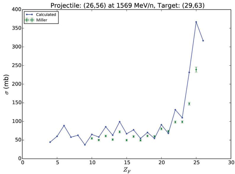
**Figure 4.52:** Elemental production cross sections (solid) compared with experimental measurements (error bars) from Ref. [29] for the reaction of  $^{56}\text{Fe}$  on  $^{63}\text{Cu}$  at 1569 MeV/A.
