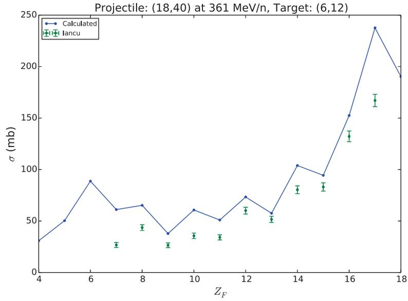
**Figure 4.43:** Elemental production cross sections (solid) compared with experimental measurements (error bars) from Ref. [18] for the reaction of  $^{40}\text{Ar}$  on  $^{12}\text{C}$  at 361 MeV/A.
