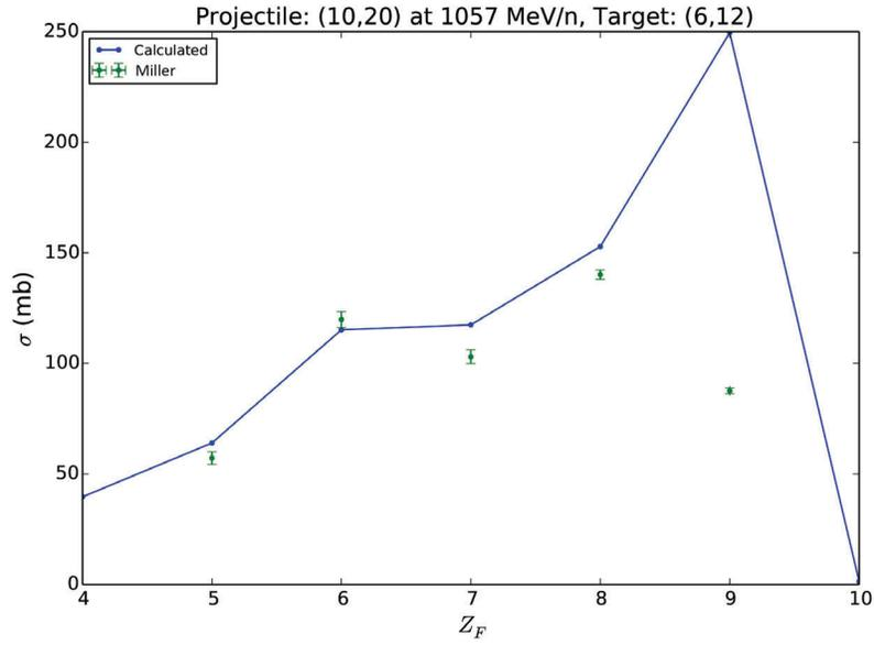
**Figure 4.17:** Elemental production cross sections (solid) compared with experimental measurements (error bars) from Ref. [29] for the reaction of  $^{20}\text{Ne}$  on  $^{12}\text{C}$  at 1057 MeV/A.
