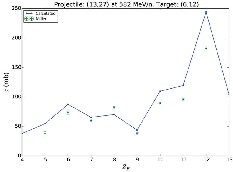
**Figure 4.19:** Elemental production cross sections (solid) compared with experimental measurements (error bars) from Ref. [29] for the reaction of  $^{27}\text{Al}$  on  $^{12}\text{C}$  at 582 MeV/A.
