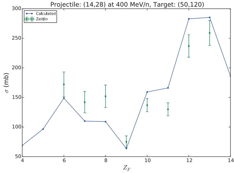
**Figure 4.23:** Elemental production cross sections (solid) compared with experimental measurements (error bars) from Ref. [52] for the reaction of  $^{28}\text{Si}$  on  $^{120}\text{Sn}$  at 400 MeV/A.
