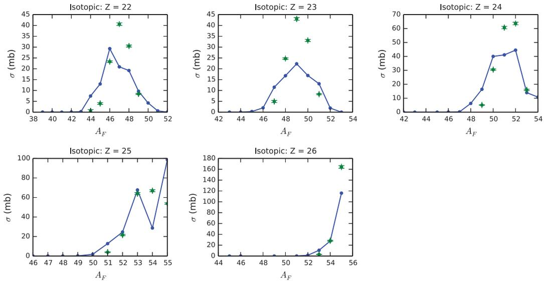
**Figure 4.59:** Isotopic production cross sections (solid) compared with experimental measurements (error bars) from Ref. [29] for the reaction of  $^{56}\text{Fe}$  on  $^{12}\text{C}$  at 600 MeV/A.
