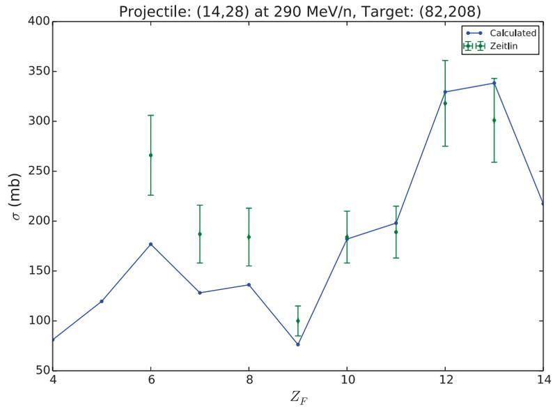
**Figure 4.20:** Elemental production cross sections (solid) compared with experimental measurements (error bars) from Ref. [52] for the reaction of  $^{28}\text{Si}$  on  $^{208}\text{Pb}$  at 290 MeV/A.
