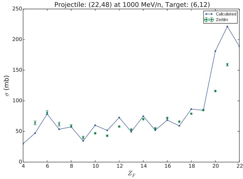
**Figure 4.49:** Elemental production cross sections (solid) compared with experimental measurements (error bars) from Ref. [54] for the reaction of  $^{48}\text{Ti}$  on  $^{12}\text{C}$  at 1000 MeV/A.
