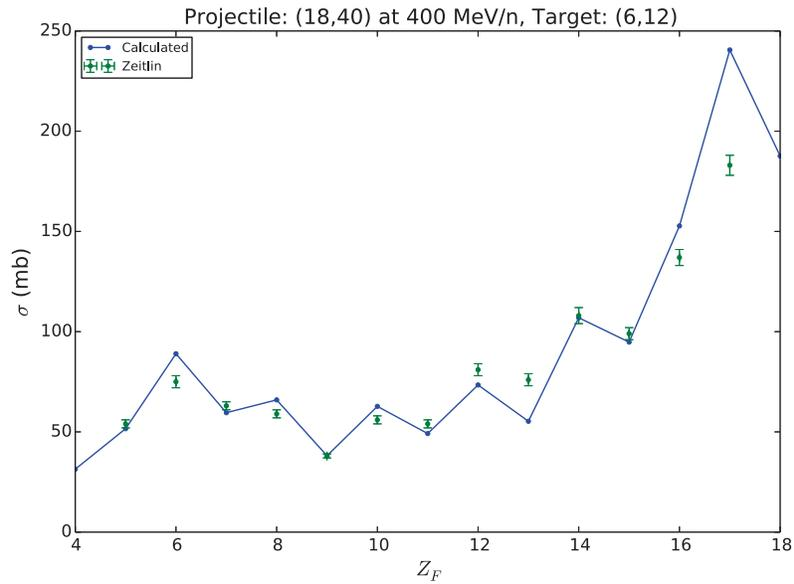
**Figure 4.44:** Elemental production cross sections (solid) compared with experimental measurements (error bars) from Ref. [54] for the reaction of  $^{40}\text{Ar}$  on  $^{12}\text{C}$  at 400 MeV/A.
