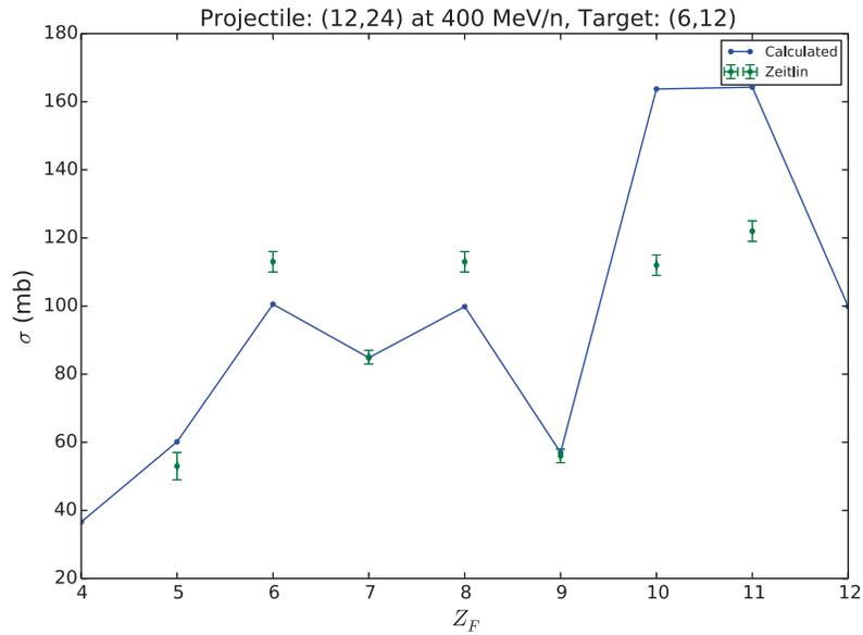
**Figure 4.18:** Elemental production cross sections (solid) compared with experimental measurements (error bars) from Ref. [55] for the reaction of  $^{24}\text{Mg}$  on  $^{12}\text{C}$  at 400 MeV/A.
