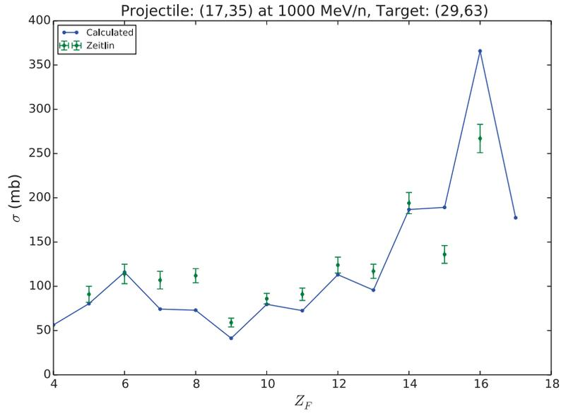
**Figure 4.31:** Elemental production cross sections (solid) compared with experimental measurements (error bars) from Ref. [54] for the reaction of  $^{35}\text{Cl}$  on  $^{63}\text{Cu}$  at 1000 MeV/A.
