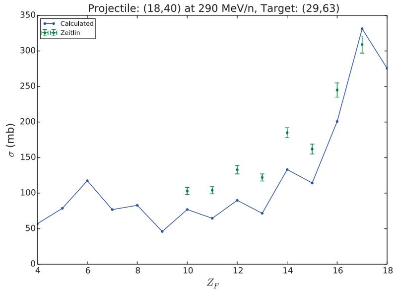
**Figure 4.40:** Elemental production cross sections (solid) compared with experimental measurements (error bars) from Ref. [54] for the reaction of  $^{40}\text{Ar}$  on  $^{63}\text{Cu}$  at 290 MeV/A.
