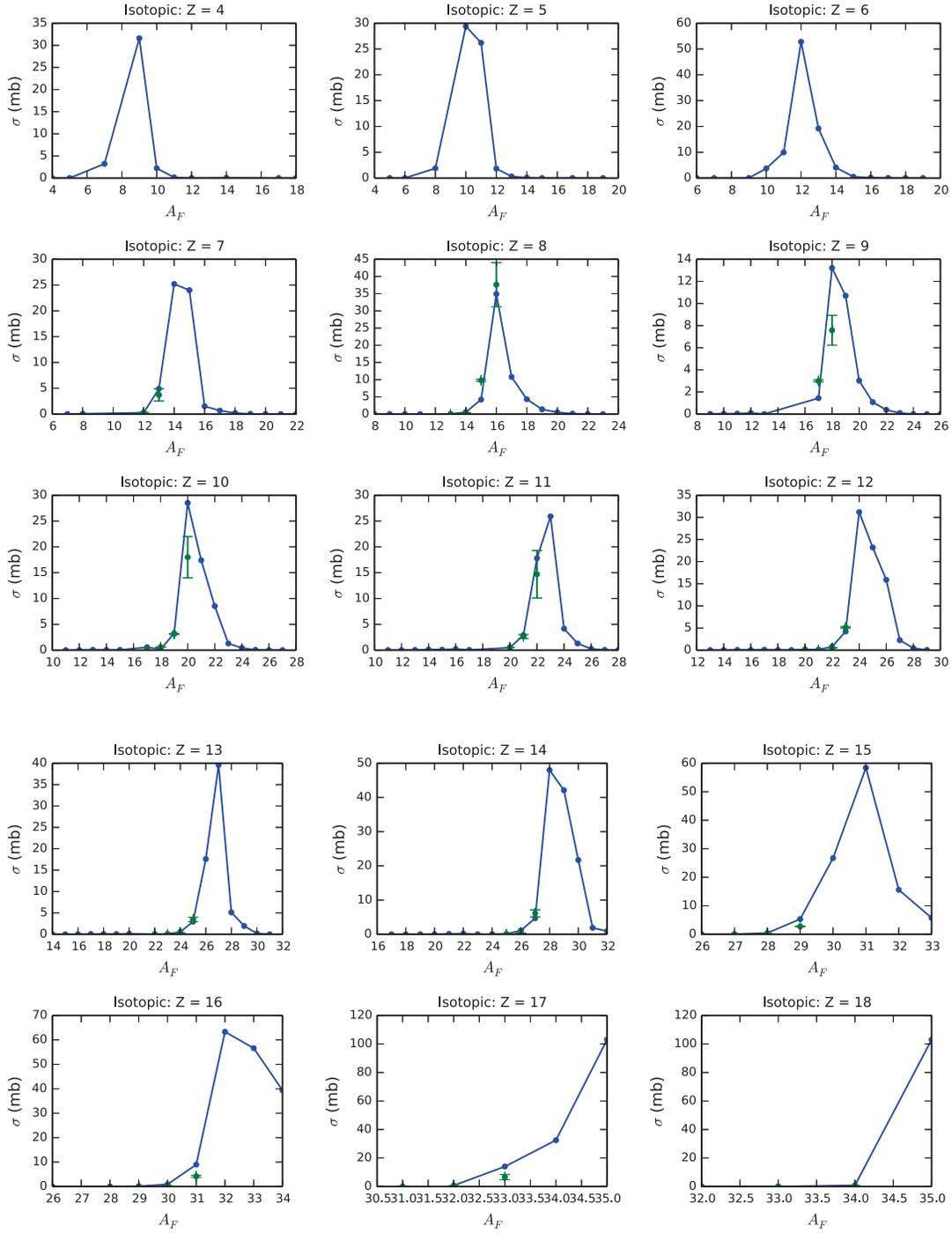
**Figure 4.55:** Isotopic production cross sections (solid) compared with experimental measurements (error bars) from Ref. [7] for the reaction of  $^{36}\text{Ar}$  on  $^9\text{Be}$  at 1050 MeV/A.
