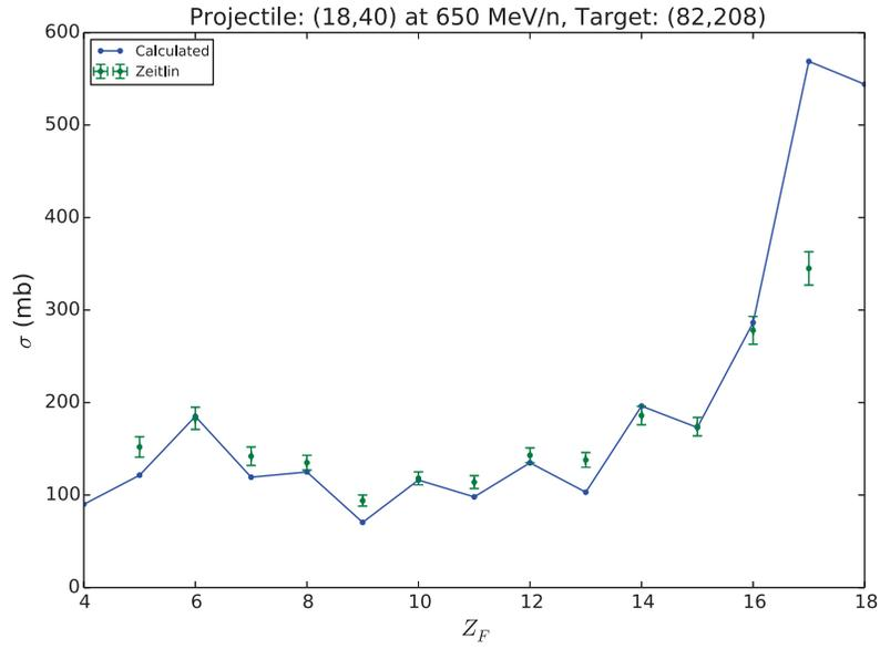
**Figure 4.47:** Elemental production cross sections (solid) compared with experimental measurements (error bars) from Ref. [54] for the reaction of  $^{40}\text{Ar}$  on  $^{208}\text{Pb}$  at 650 MeV/A.
