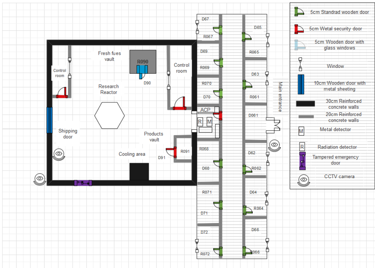
Figure 4: The New Research Reactor Building Floor Plan
