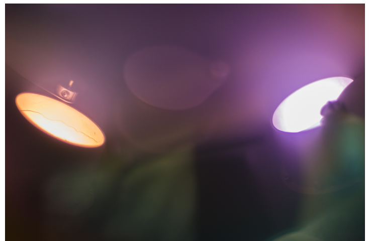
Figure (6) - The interior of the sputtering chamber. The orange target on the left is Au and the purple target on the right is Ni..
