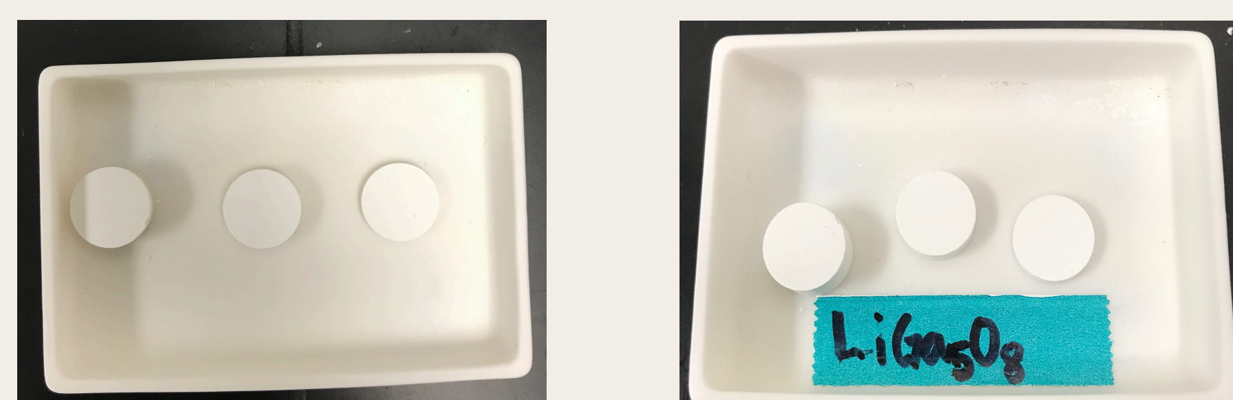
Fig. 1: On the left is \text{LiGa}_5\text{O}_8 before sintering, and on the right is after sintering
