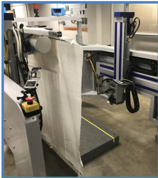
Figure 24: Back view of the white sheet draped over the x-ray emitter axis.
