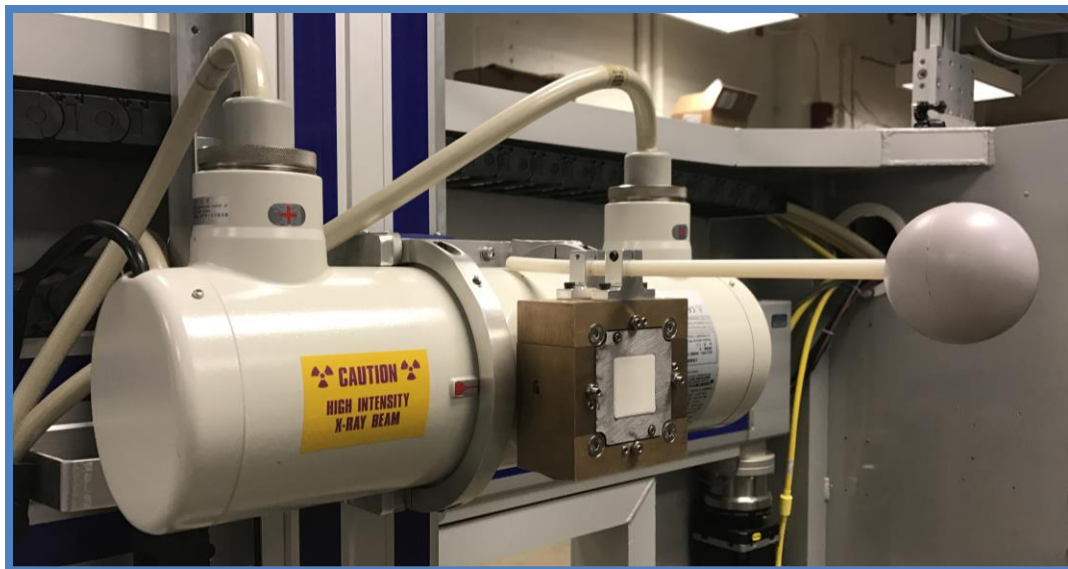
Figure 4: Toshiba X-Ray Emitter with distance standoff rod.
