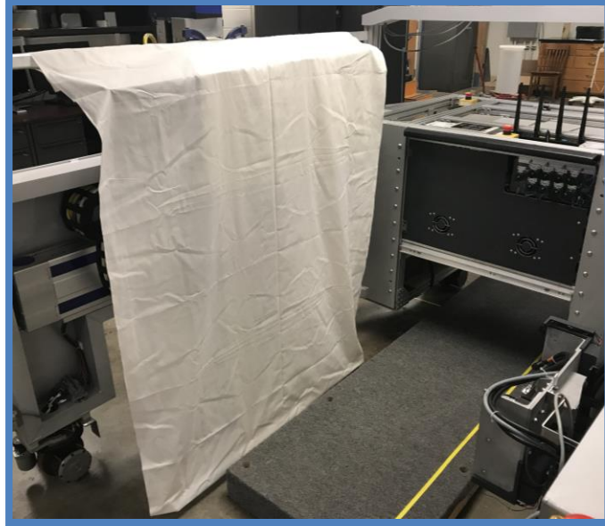
Figure 23: White sheet draped over x-ray emitter axis to simulate the light background of an x-ray image.
