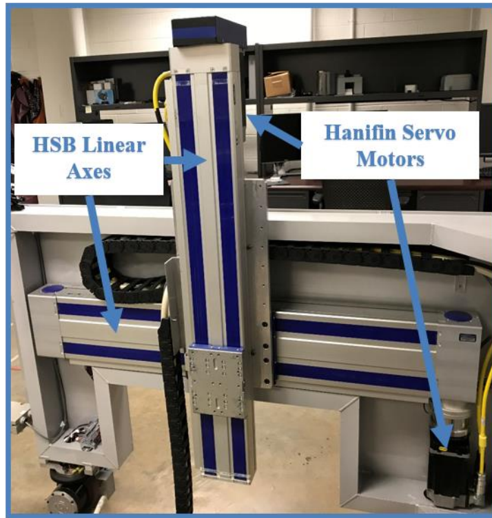
Figure 7: Horizontal and Vertical Schunk Axis Drives for x-ray system motion.
