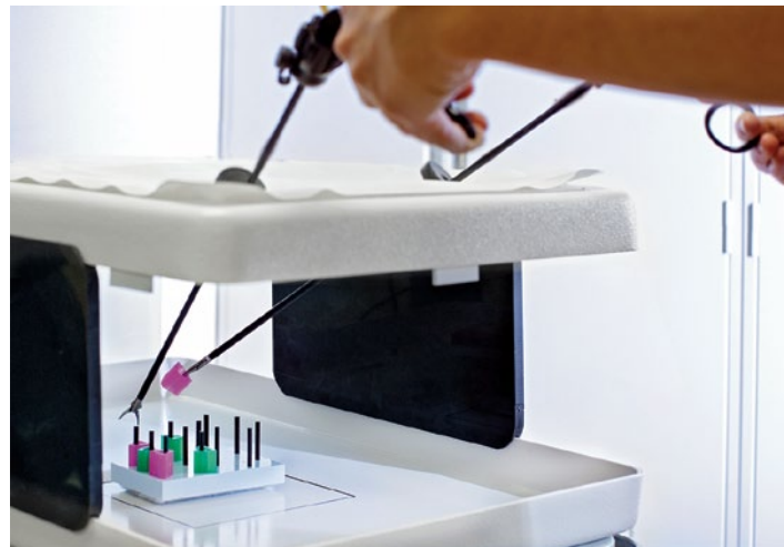
Tools such as the laparoscopic box trainer are used in the simulation center to practice fundamental laparoscopic surgical skills.
