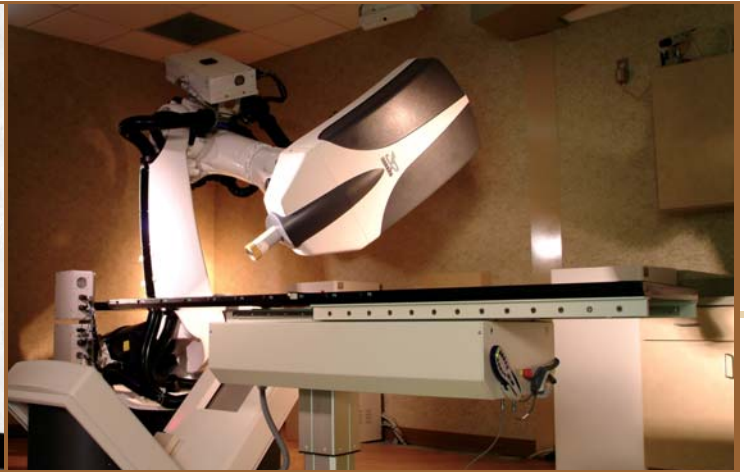
CyberKnife generates and delivers radiotherapy to treat tumors in the brain and other soft tissue such as the liver and lungs.
