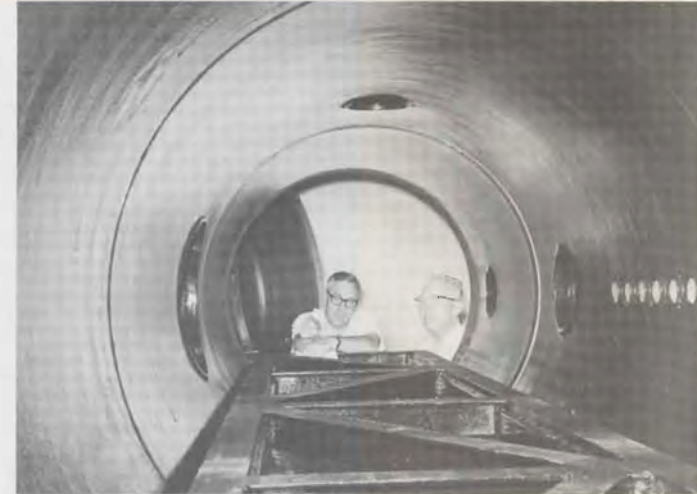
U-T physicists examine an instrument chamber for an infrared spectrometer, to be used in studying atmospheric gases of other planets.
