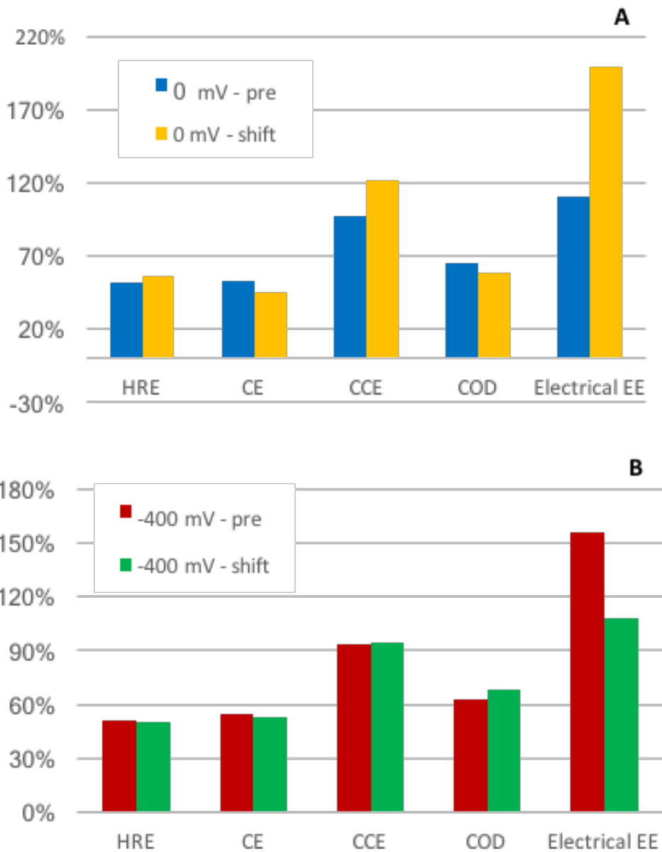
Figure 48: Efficiency values for pre and post potential (A) 0 mV reactor shifted to -400 mV and (B) -400 mV reactor shift to 0 MV.
