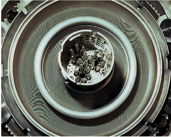
Figure 6 Top of the inner and outer fuel elements as well as the target bundle [13]
