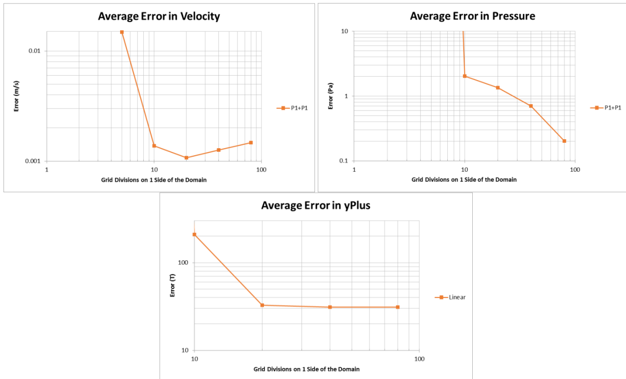
Figure 135 Average error in velocity, pressure and yPlus for Eca yPlus turbulent case plotted against grid refinement
