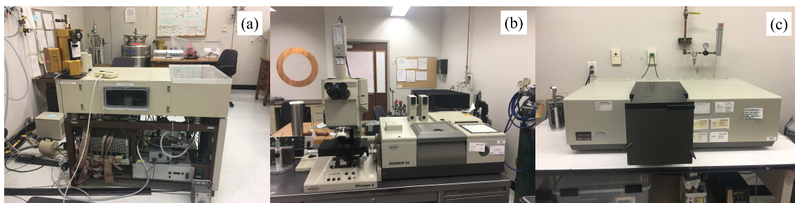
Figure 3.1: Infrared spectrometers employed for work presented here. (a) Bruker 113v and (b) Bruker Equinox 55 Fourier transform spectrometers, and (c) Perkin Elmer Lambda-900 grating spectrometer.
