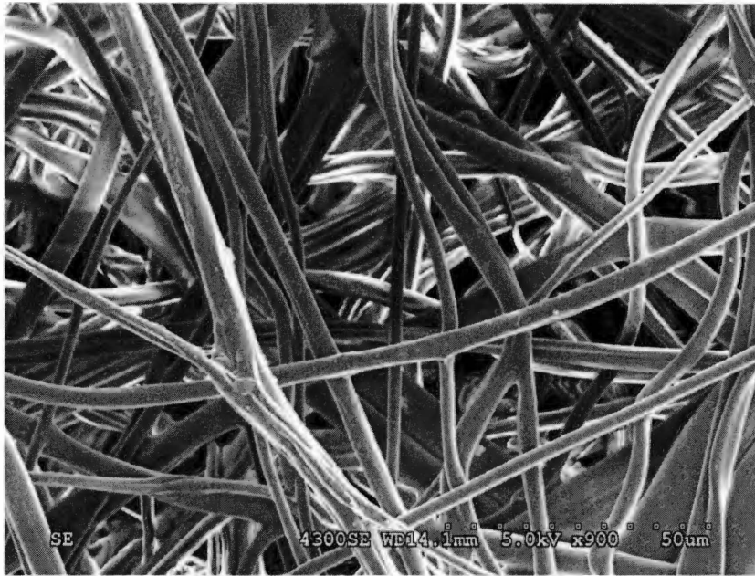
Figure 3.18 SEM photo of sample 1 (75PE/25PA) before heat stretching treatment
