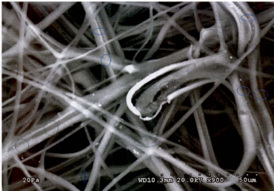
Figure 4.4 50PBT/50PP MB web after treating with 16.7% NaOH for 45 min
