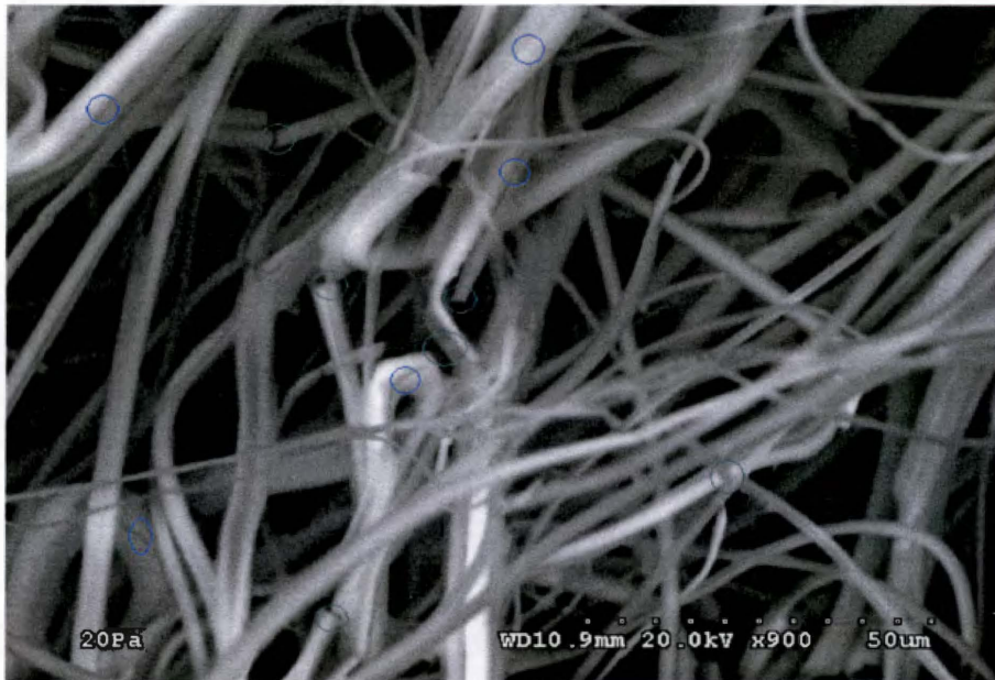
Figure 4.1 50PBT/50PP MB web after treating with 16.7% NaOH for 3 min
