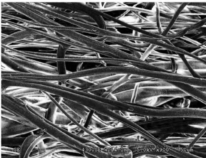
Figure 3.19 SEM photo of sample 1 (75PE/25PA) after heat stretching treatment
