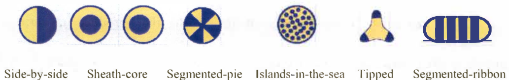
Figure 1.2 Cross-sectional conformations of different types of bicomponent fibers
