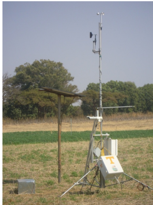
Figure 2. Micrometeorological station with rotating arms at the Mt. Pleasant, Zimbabwe study site
