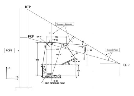
Figure 2 Clearance distance shown relative to the SAE J2194 clearance zone. Dimensions in millimeters.
