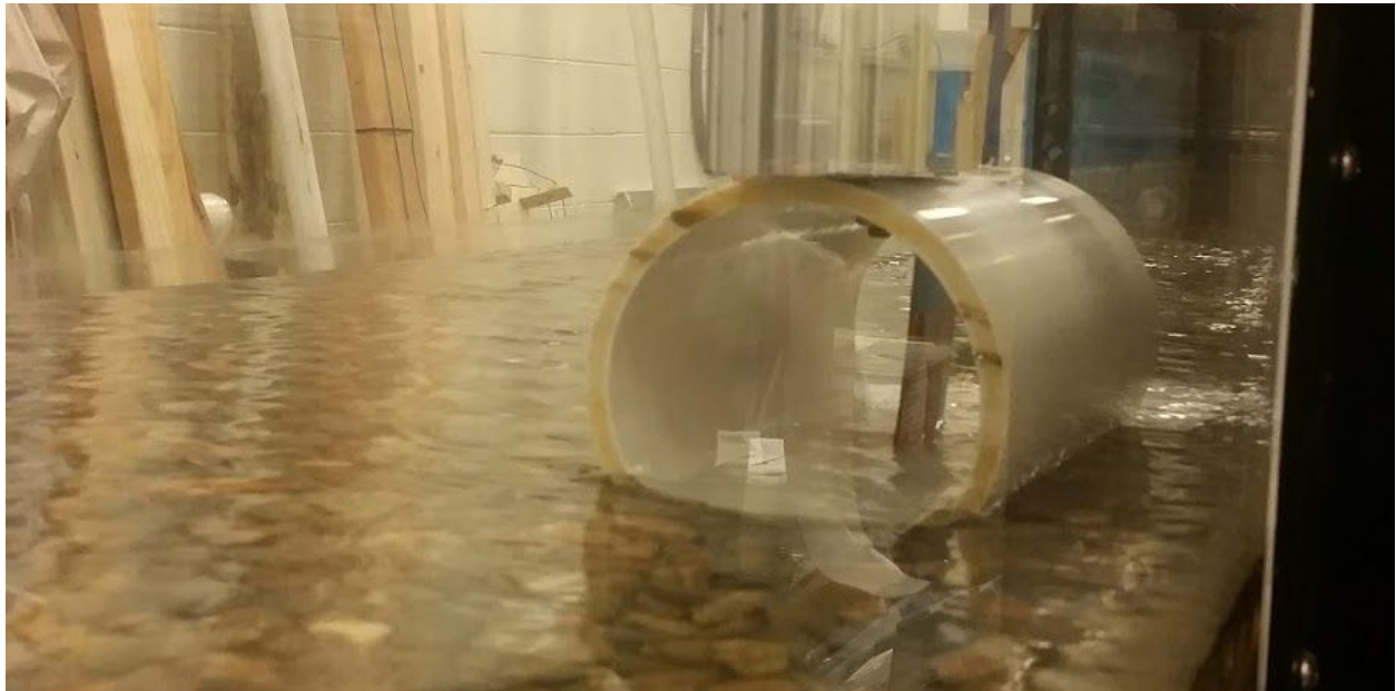
Figure 1: The section of tile used in the H&S Lab to test our final sensor.
