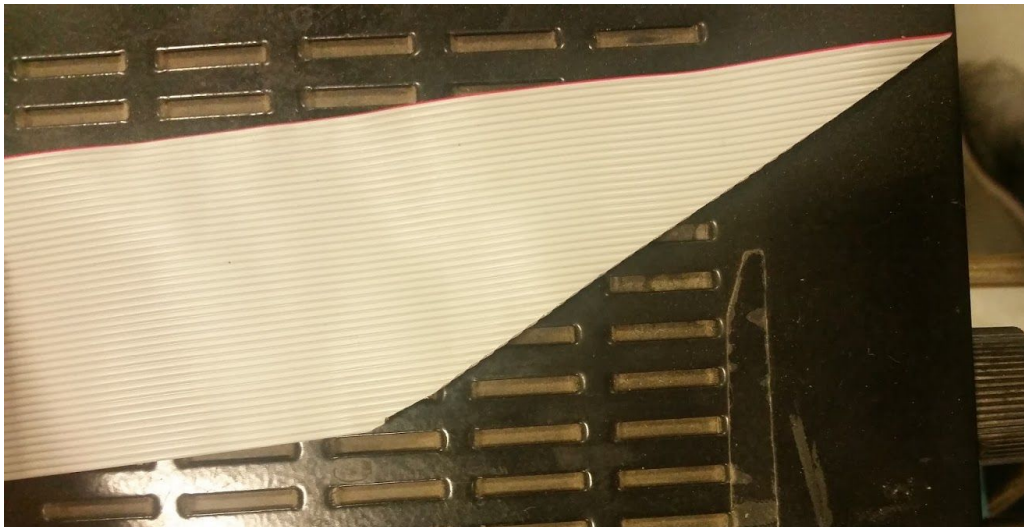
Figure 1: The ribbon cable used for the electrode sensor. Note the diagonal cut that demonstrates our ability to allow variable resolution in the tile.
