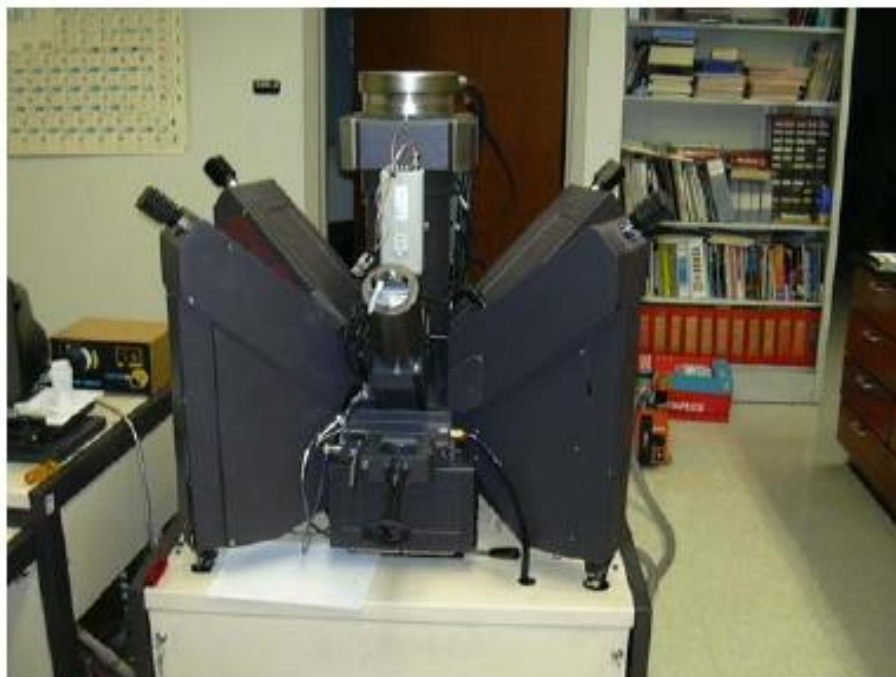
Figure 3.5.1 Cameca SC-52 EPMA device [17, p. 58].
