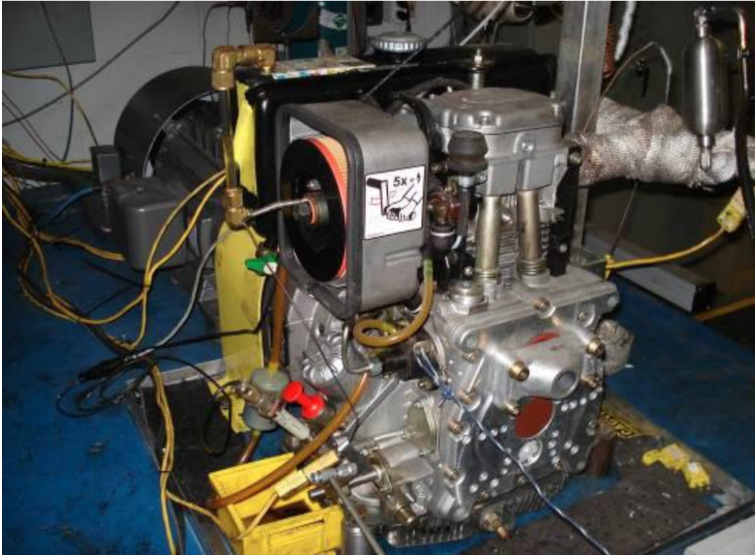
Figure 3.2.1 Single-cylinder Hatz diesel engine for accelerated Na-aging protocol [1, p. 44].
