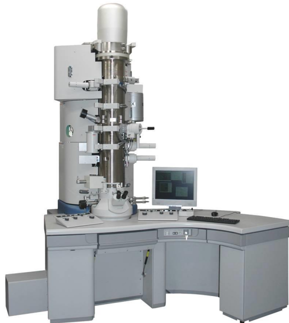
Figure 3.5.2 TEM used for fresh and engine-aged LNT analysis.
