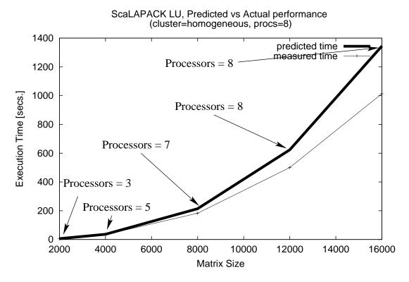
Figure 2.4: Validation of execution model on a homogeneous cluster for different matrix sizes
