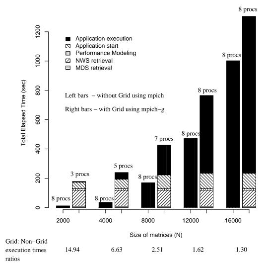
Figure 2.7: GrADS overhead on a homogeneous cluster
