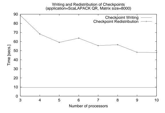
Figure 5.14: Times for Checkpoint Writing and Redistribution when the application was restarted on different number of processors
