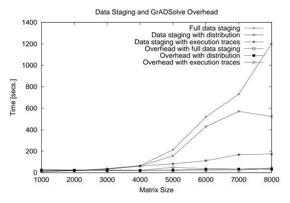
Figure 6.9: Data staging and other GrADSolve overhead
