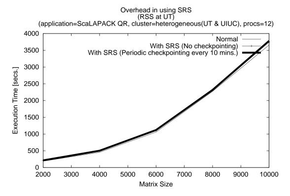
Figure 5.11: Overhead in SRS on a heterogeneous cluster
