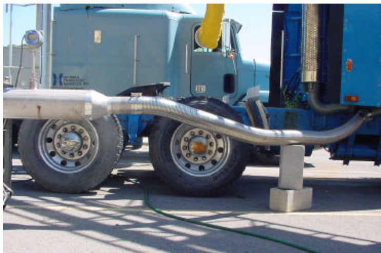
Figure 3.2. Test truck attached to primary sampling chamber.
