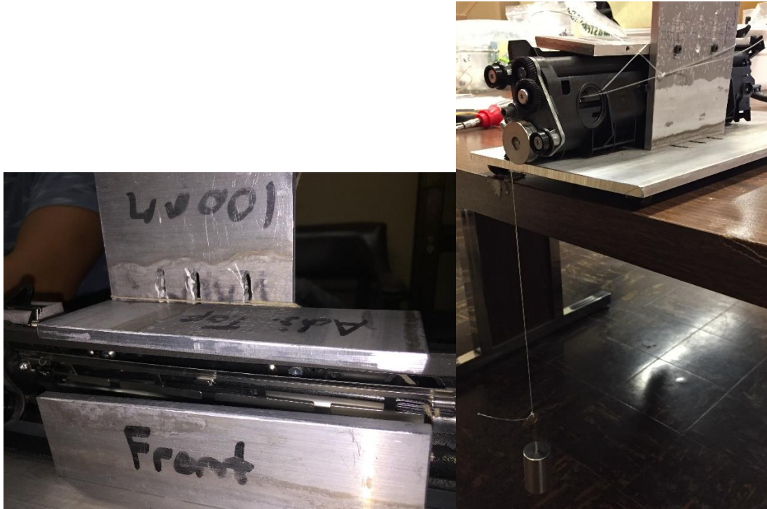
Figure 5. Gear Failure Test Apparatus and Loading Flywheel
