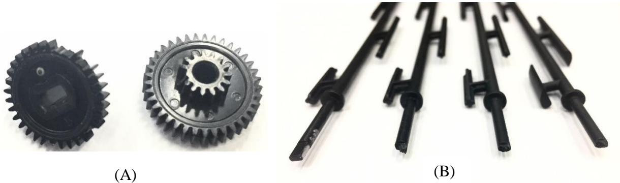
Figure 9. Gear Failure Test Failure Modes with (A) Molded Gear Failure and (B) Molded, Old Design Machined, and New Design Machined Agitator Shaft Failure
