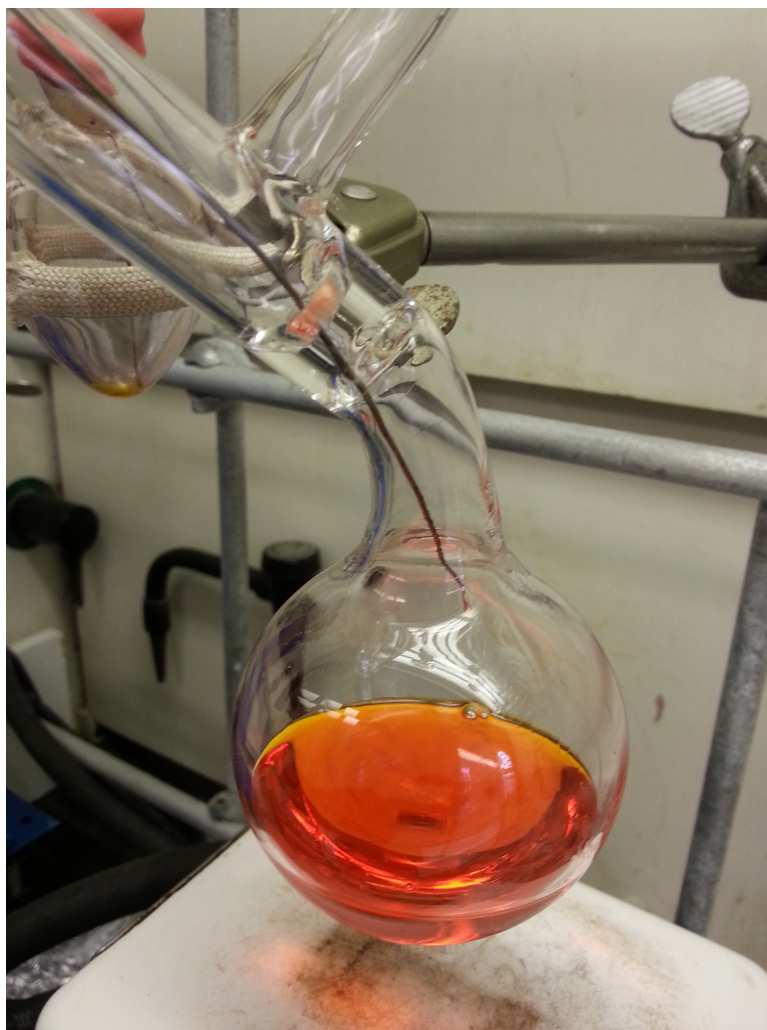
Figure A.1: Schlenk flask used for hydrosilylation reactions that is fabricated from heavy boiling flasks.
