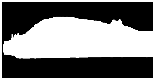
Figure 4.11: Result of applying median and dilation filters to the segmentation in Fig. 4.10.
