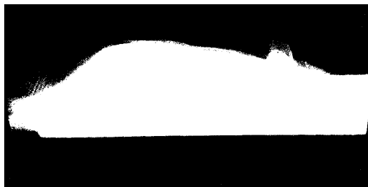
Figure 4.10: Initial segmentation of the projection from Fig. 4.9 using a threshold value of 98%. This segmentation contains some salt and pepper noise.
