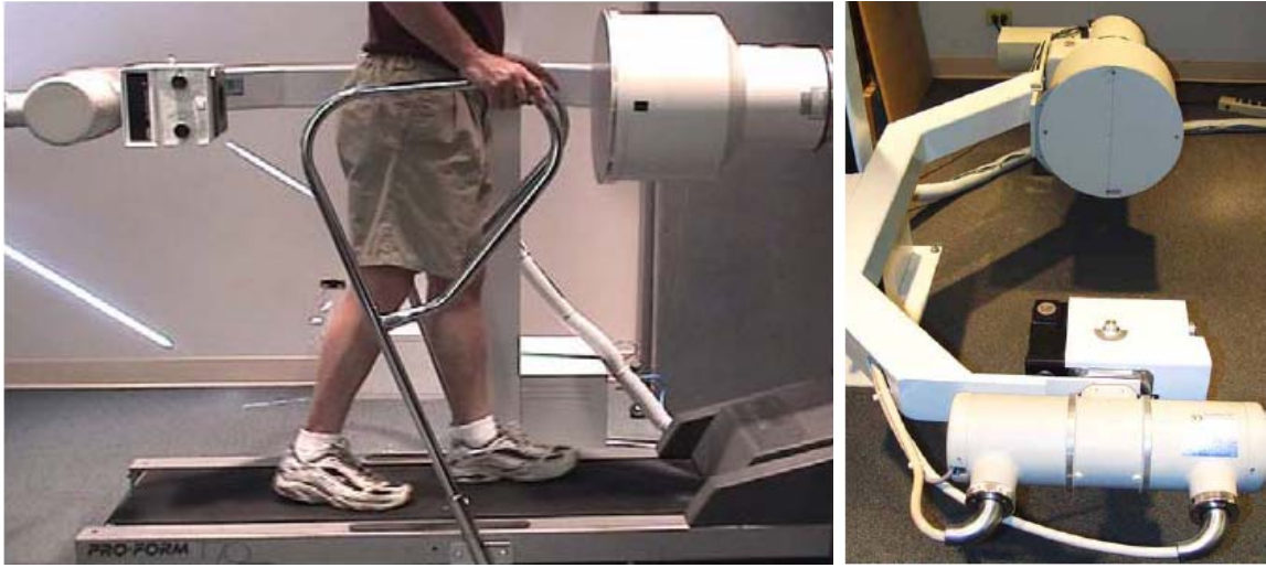
Figure 5: Fluoroscopy Machine with Treadmill and Subject [left]; Top View of Fluoroscopy Machine, Image of Radiation Source to Image Intensifier [right]
