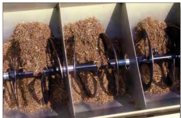
Fig. 5.23 and 5.24 Drills with “picker wheels” and agitators in the seed box (such as this Truax™) are recommended when planting bluestems and indiagrass. This ensures an even flow of seed and prevents seed lodging in the box.
