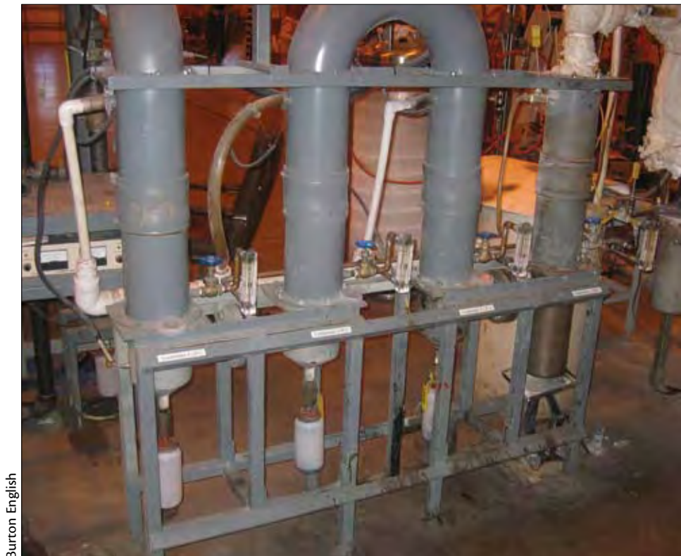
Fig. 4.2 This pyrolysis unit is responsible for converting plant matter into bio-oil using heat in the absence of oxygen.
