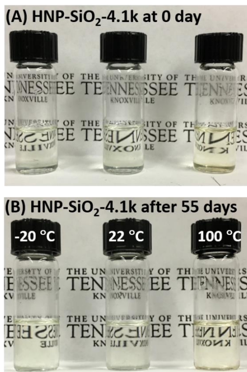
Figure 4.7. Photos of 1 wt% dispersions of HNP-SiO 2 -4.1k in PAO in the initial state (A) and after being kept at -20, 22, 100 °C for 55 days (B).
