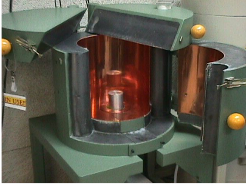
Figure 4.1: HFIR-NAA Facility Graded Shield with HPGe Detector
