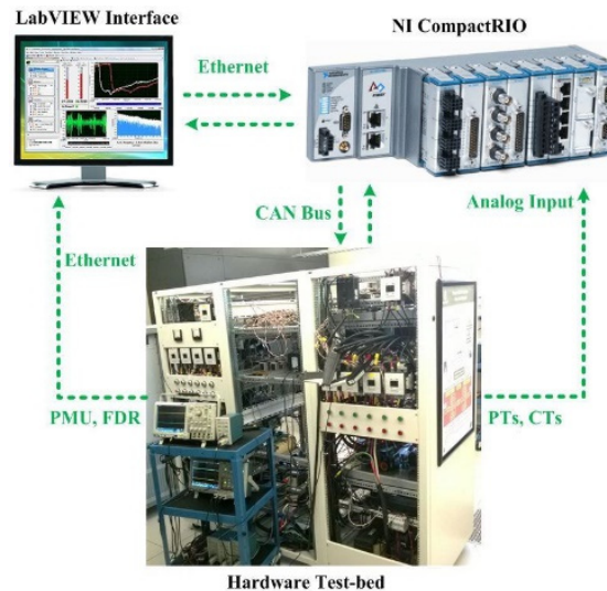
Figure 56. HTB control and communication structure.
