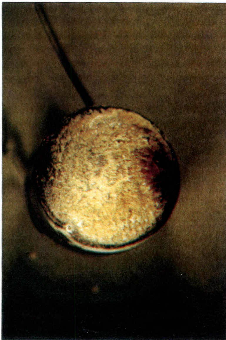
Figure 4.5.4. Photograph of reacted pellet from Run 227, prepared at 550°C, 30 min, 2000 pm HCl.
