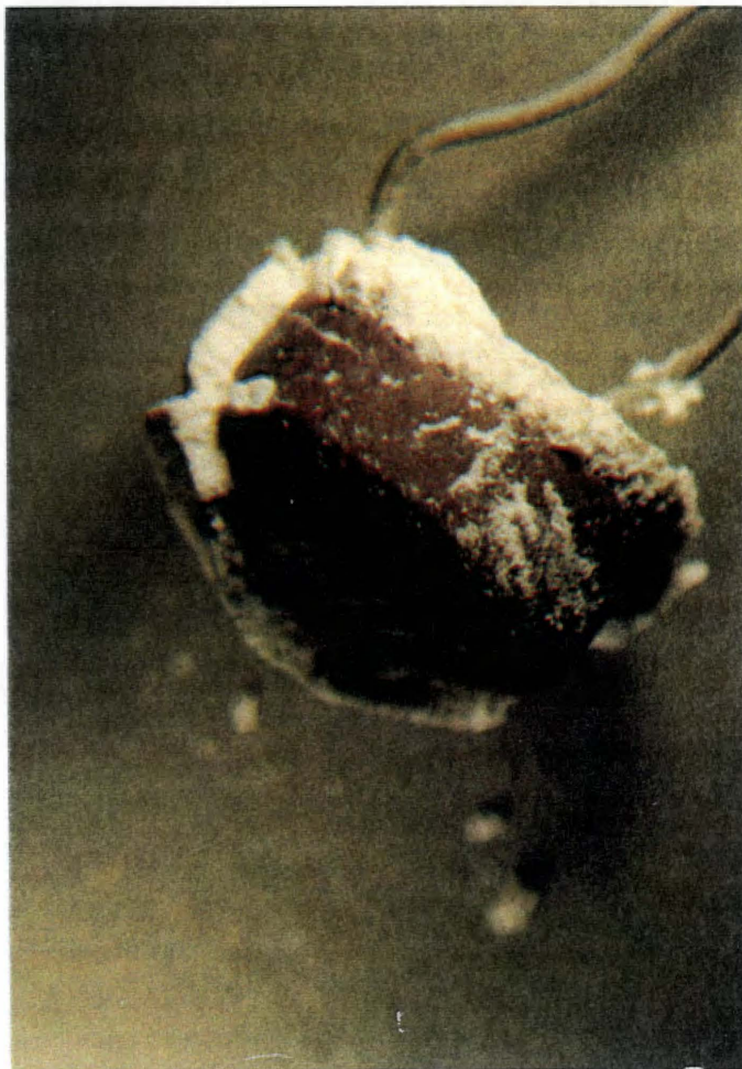
Figure 4.4.3. Photograph of pellet from Run 306, prepared at 328°C, 115 min, 4000 pm HCl.
