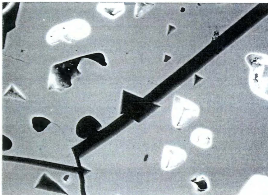
Figure 4.6.13. Electron micrograph at 1000x of middle of ash layer of pellet from Run 245, prepared at 670°C, 60 min, 2000 ppm HCl.
