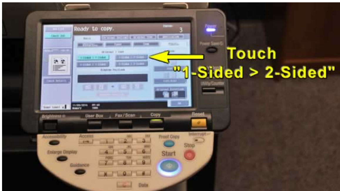
Figure 4.18: Example image annotated with text and instructions pushed to the Google Glass AR device for step 5 in the copy machine study.
