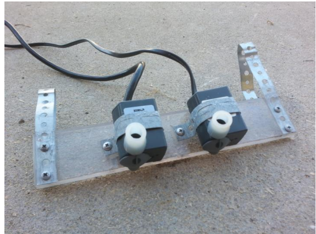
Figure 18. First generation sample chamber pumps.
