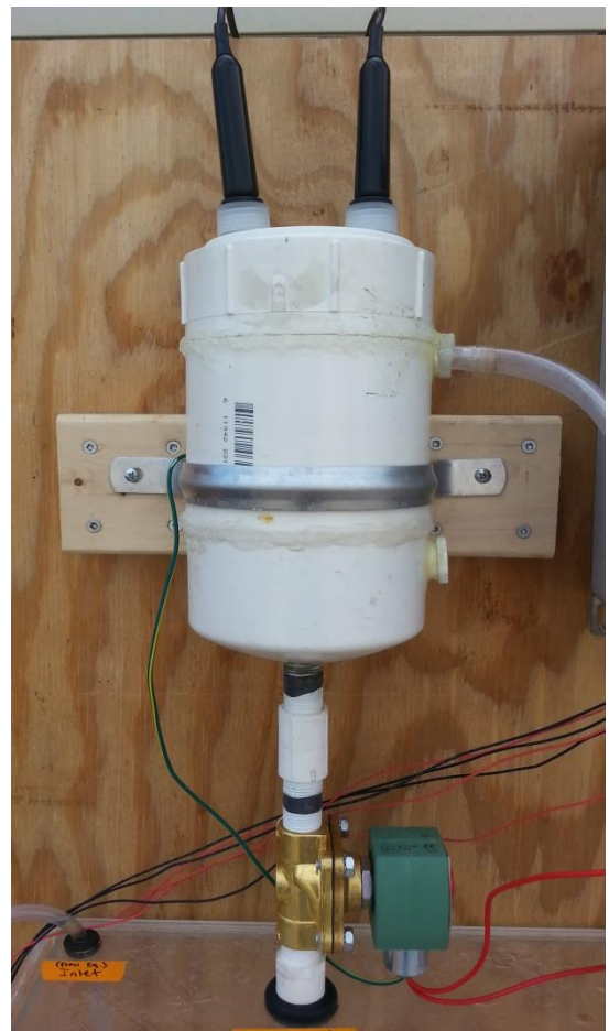
Figure 16. Ammonium and Nitrate Sample Chamber.
