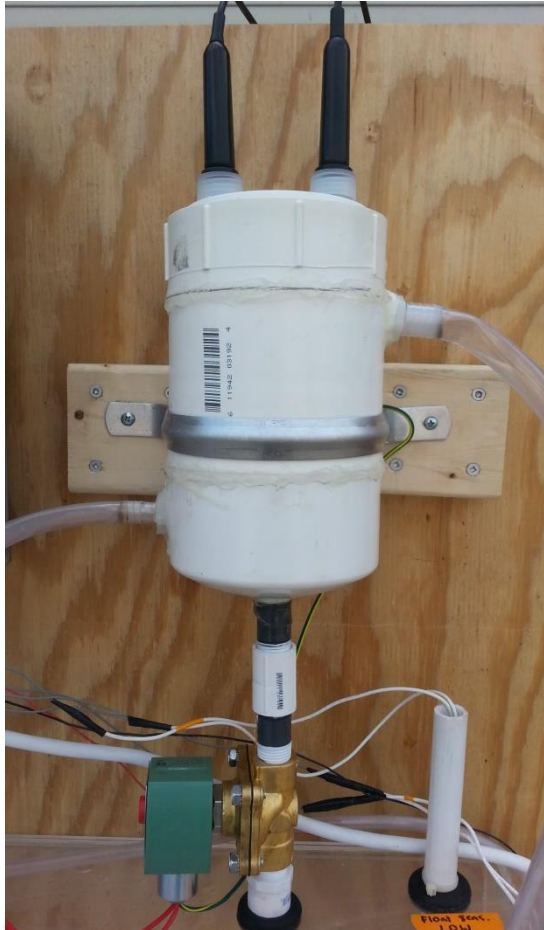
Figure 17. Dissolved Oxygen and pH Chamber.
