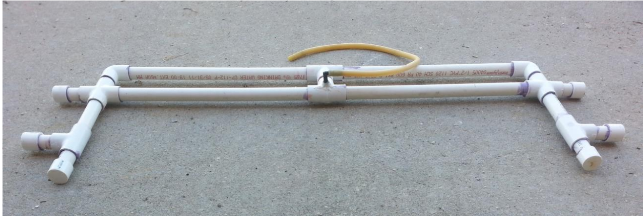
Figure 21. Second generation sequencing batch reactor decanter.
