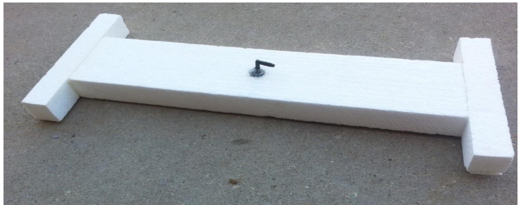
Figure 20. First generation sequencing batch reactor decanter.
