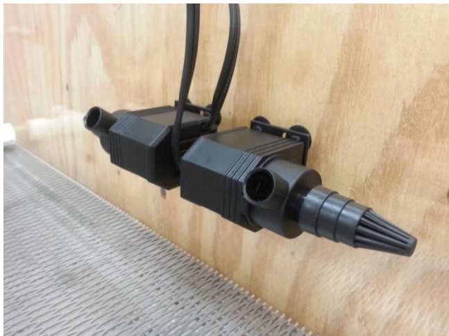
Figure 19. Second generation sample chamber pumps.
