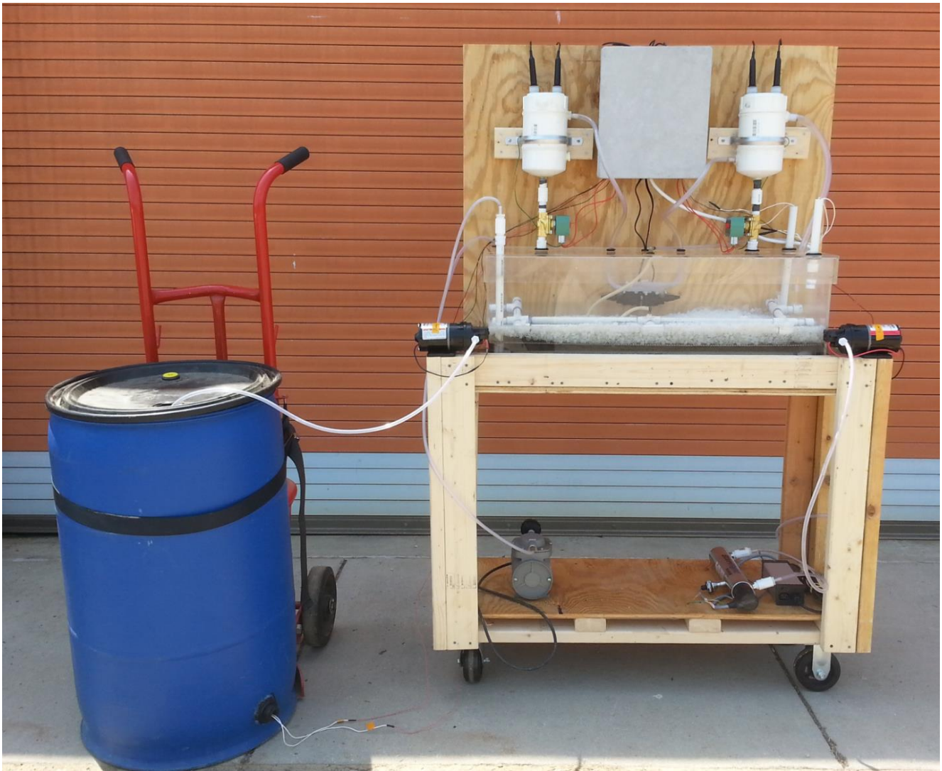
Figure 11. Image of laboratory scale flow equalization tank, sequencing batch reactor, and disinfection.
