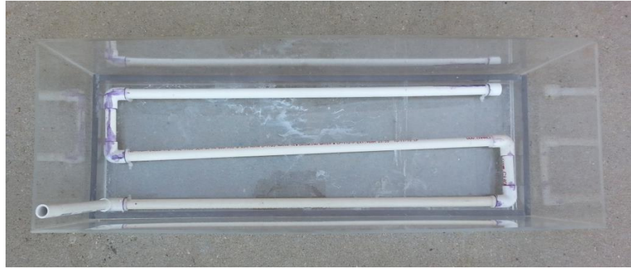
Figure 14. Aeration piping attached to the SBR tray.
