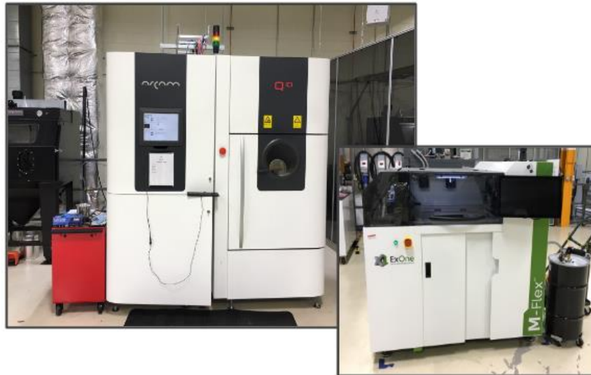
Figure 2.4: Arcam Q10 AM Machine (Left) and M-Flex ExOne AM Machine (Right)
