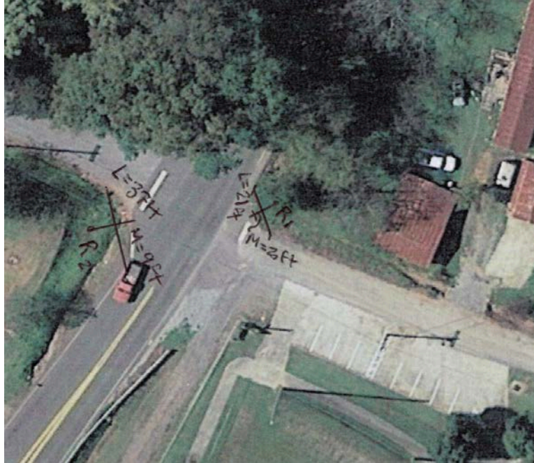
Figure 4.3 Existing Curb Radii
