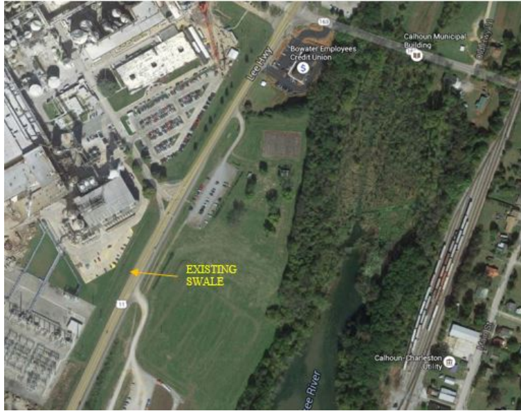
Figure 3.2: Existing Stormwater Management, Highway 11
