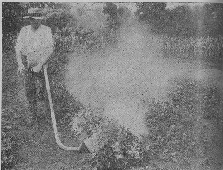
Rotary dust gun, showing manner of turning nozzle sideways to direct dust to underside of leaves
