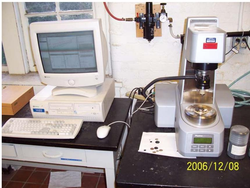
Figure 5.5 Anton Paar Physica MCR 501 Rheometer
