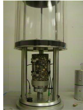
(b) Specimen placed in the confining pressure chamber
