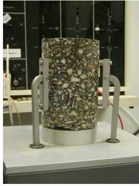
(a) Studs attached to specimen
