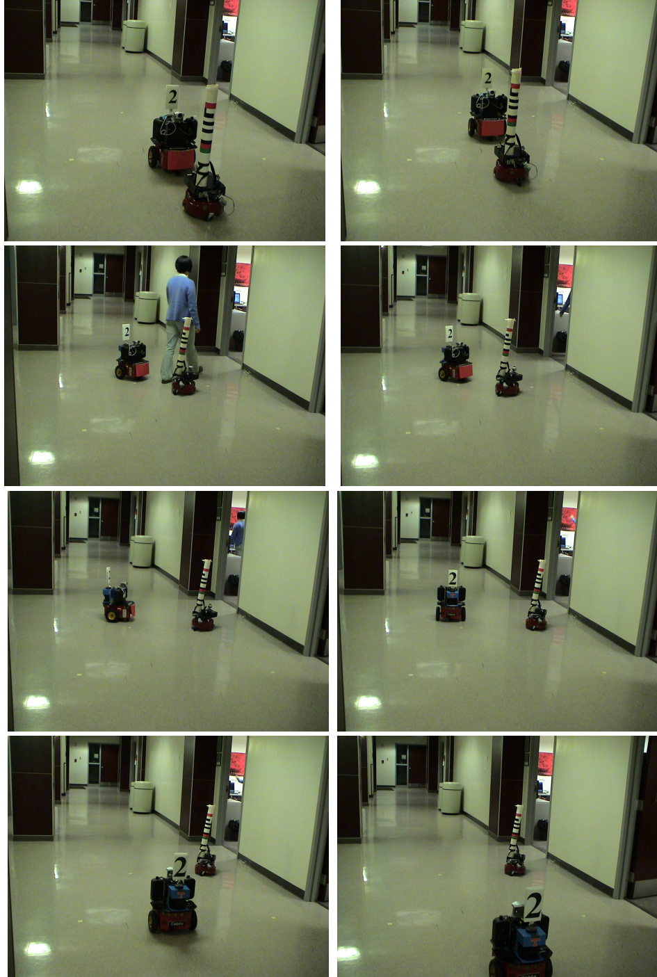
Figure 6.16: Deployment of a sensor robot using assistive navigation: the lead robot reaches a pre-specified way-point, tele-operators the sensor robot into position and heads back to the starting position (read left to right, top to bottom).
