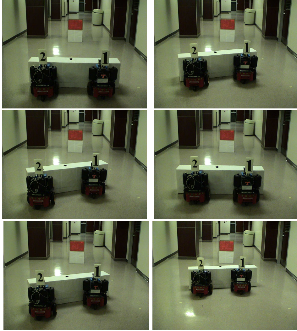
Figure 6.2: Example of a box pushing task – Robots 1 and 2 push a long box towards the goal indicated by a blob at the far end of the corridor. Robot 1 pushes one end of the box and waits until robot 2 has successfully pushed its end. The process continues until the goal is reached (read left to right, top to bottom).
