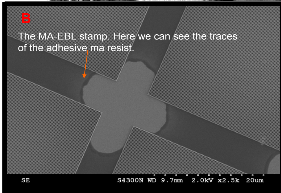
Figure 3.15 (a) SEM micrographs of PDMS substrate shows that some discs were transferred but not sufficient for SERS application (b) SEM micrographs of EBL stamp of ma-N2403 resist after developing the patterns.
