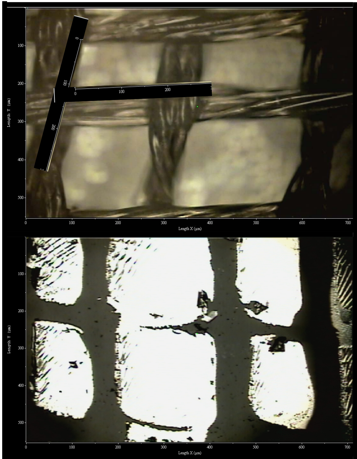
Figure 3.5 (Top) White light illumination of the original mask with dimension of squares being 200\ \mu\text{m} \times 200\ \mu\text{m} . The bottom is the white light illumination of the macro-Ag pillars transferred onto PDMS.
