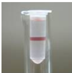
Figure 5.12: Forward extraction of cytochrome c by 1 wt.% of overall surfactant at 25°C using the conditions listed in Figure 5.9 .
