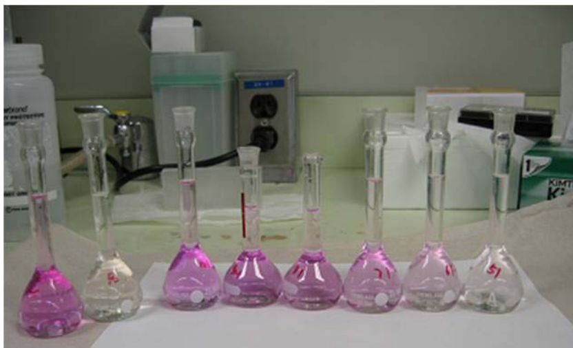
Figure 2.5 The effect of indicator on color change in chromium solutions
