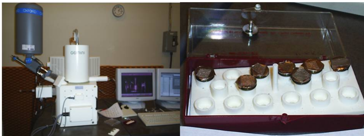
Figure 2.4 FESEM - LEO 1525 (left), gold sputter coated electrospun fiber samples for SEM imaging (right).
