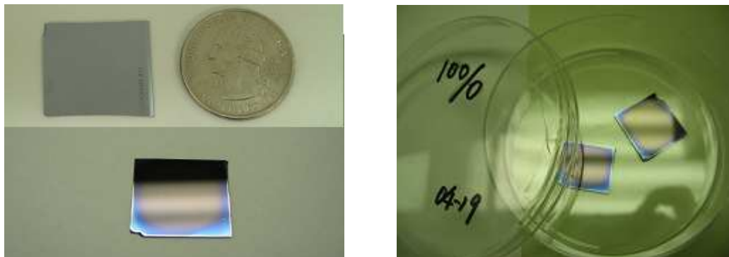
Figure 5.2 Photographs of ultra-thin chitosan films prepared by placing 0.5 ml chitosan solutions on the silicon chips and spun using a spin coater at spin speed of 2500 rpm for 60 seconds. The size of film with silicon chip was compared to a quarter.
