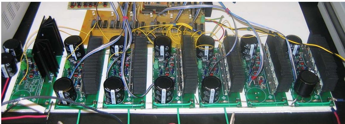
Figure 7-19. The proof of concept; the 6-level 5 kW MMCCC with 6 modules. The sixth module (first one from right) is bypassed for normal operation.
