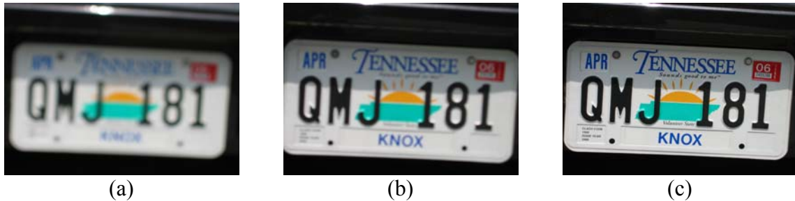
Figure 7.2. Sample images from the LP sequence (system magnification: 2.28\times , target distance: 1m): (a) far focus end, (b) near focus end, and (c) best focus.
