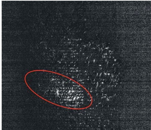
Figure 68 Thermal image of a soldering iron recorded with SiO 2 deformation-magnification FPA at atmospheric pressure
