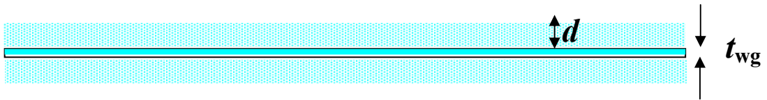
Figure 3.6 A) Bulk optical planar waveguide regime. B) Integrated optical waveguide regime. t_{wg} denotes the waveguide thickness, with d representing the depth of the evanescent wave.
