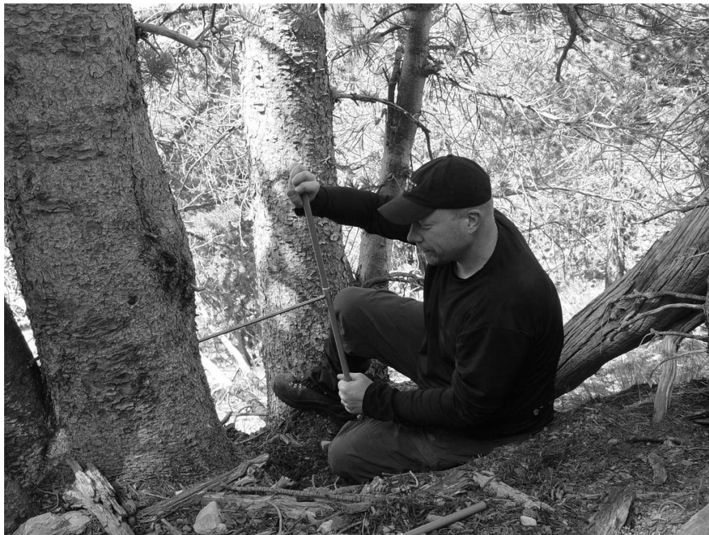
Figure 3.2. Collecting cores with an increment borer from whitebark pine at the Western Beaverhead site.
