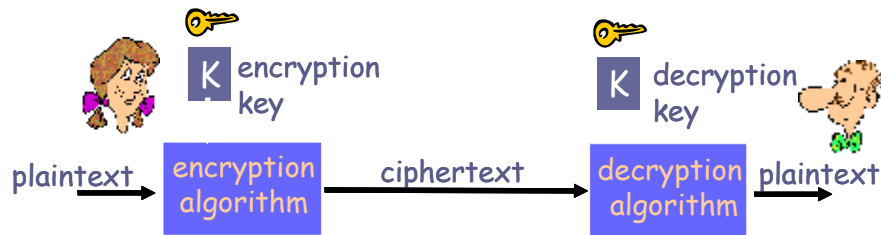
Figure 2-1: The foundations for symmetric cryptography: Alice is encrypting the plain message, and Bob is decrypting the ciphertext, while both use the same shared secret key (redrawn from [42])
