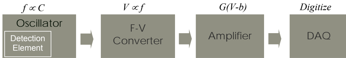
Figure 33. Functional diagram of sensor circuitry and data acquisition system
