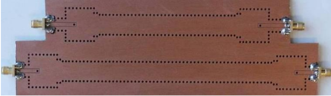
Figure 4.6 Back to back transitions with different lengths for insertion loss measurement.
